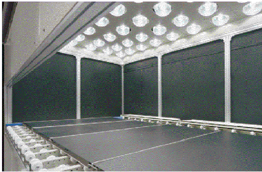
Solar simulator interior: The open chamber of this multi-lamp fixed light simulator makes it easy to insert and remove PV modules.
