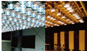
Dual Technology Lighting System (Combined Metal Halide and Halogen Technology) Ideal for custom environmental testing such as vehicle performance evaluation and artificial climate chambers.
