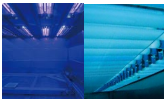
Ultraviolet Lamps Spectral distribution corresponding to PV qualification standards (IEC61215 / IEC61646).
