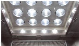
400W Metal Halide technology Lamp Complies with IEC and JIS Class C spectrum conformity.
