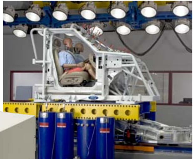
High speed photography applications demand extreme light stability to achieve high resolution along with the required depth of field.
